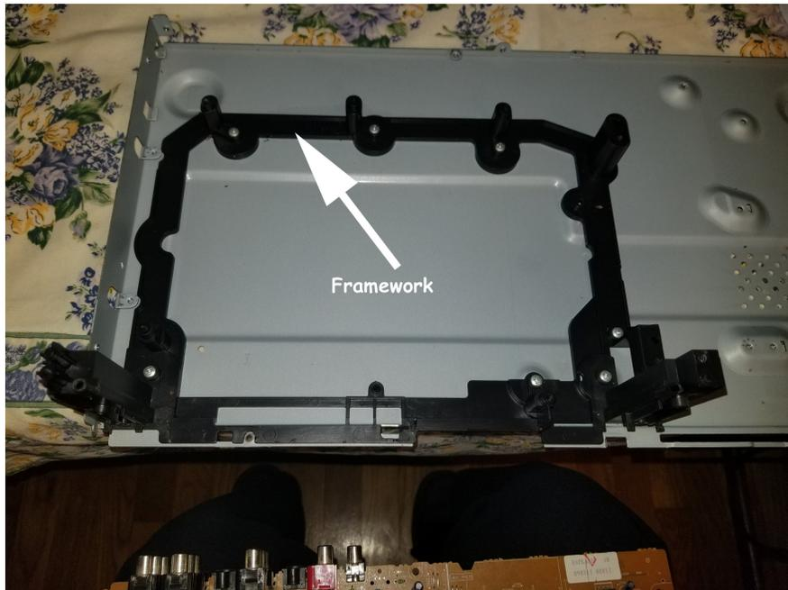
Fig. 20 – Case bottom and framework after circuit board/VCR removed
