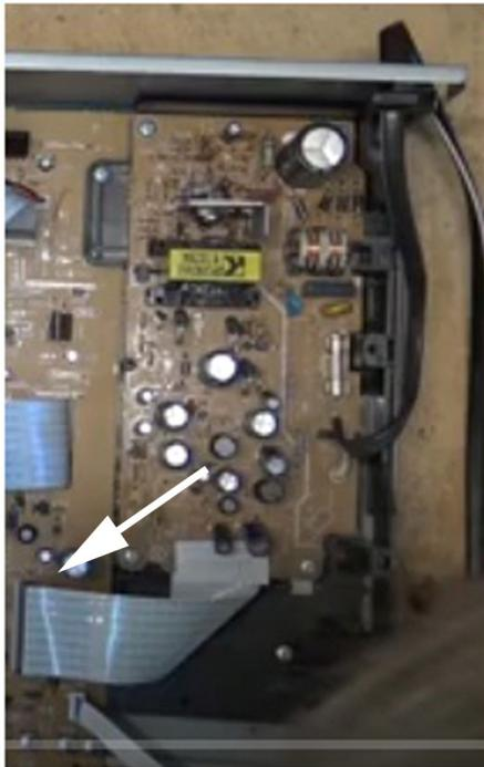
Fig. 12 – Slip out ribbon cable from circuit board
