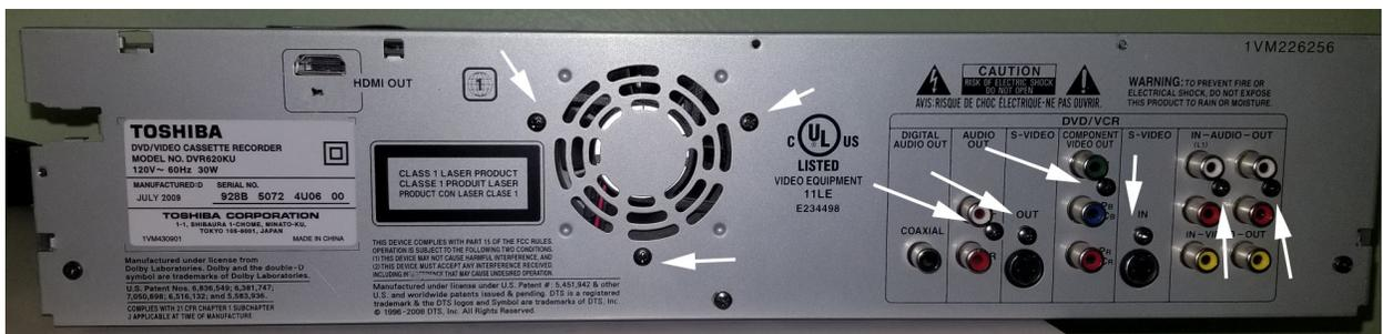
Fig. 14 – Back panel showing 9 screws
