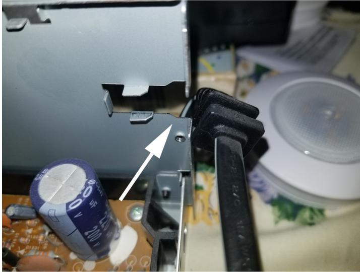
Fig. 11 – Slide power cord out of back panel
