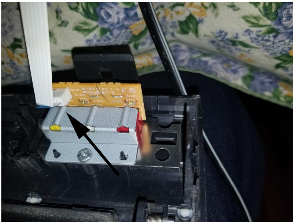
Fig. 5 – Slide out ribbon cable from front panel
