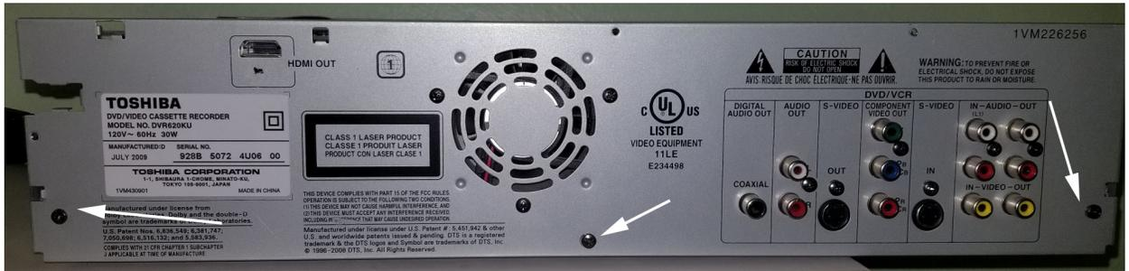
Fig. 15 – Three screws to remove to separate back from bottom case
